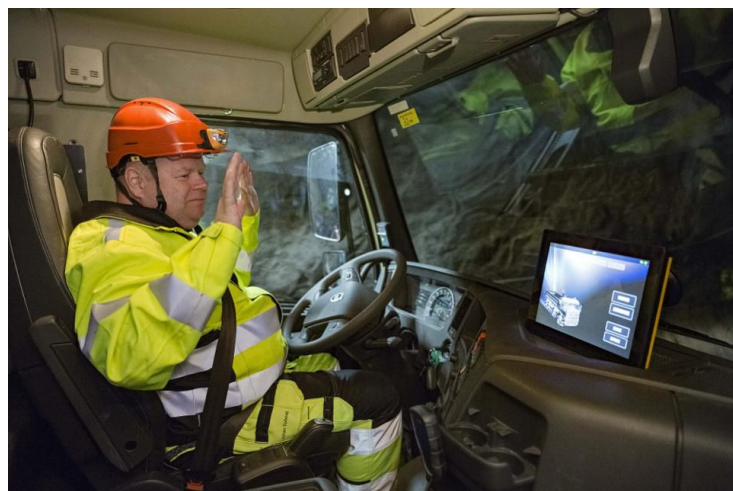
A driver lifts his hands away from the steering wheel of a Volvo Autonomous FMX self-driving truck, manufactured by Volvo Group, as it drives through underground tunnels, at Kristineberg mine in the Boliden area in Arvidsjaur, Sweden, on Friday, Sept. 2, 2016. The Autonomous FMX is equipped with LiDAR light radar sensors and GPS technology to create 3D maps of the vehicle's surroundings enabling it to navigate its way through tunnels. Photographer: Krister Soerboe/Bloomberg
