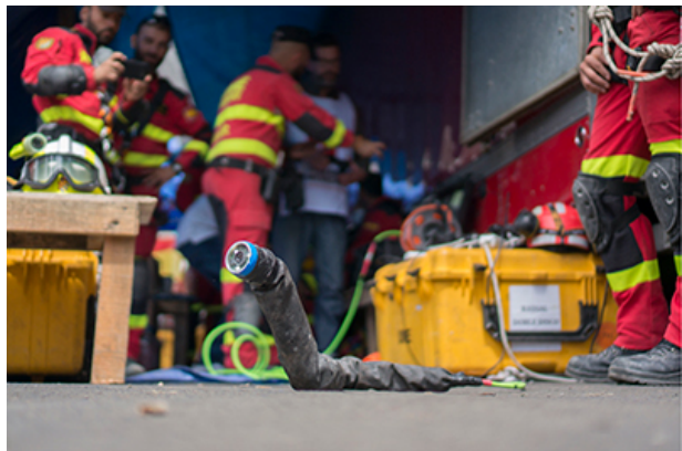
Snake-like robot helps first responders with search and rescue efforts by maneuvering into tight spaces and accessing difficult-to-reach areas. (Courtesy of Carnegie Mellon University)
